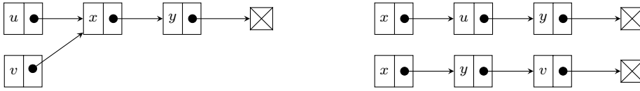
Fig. 7: Term representation w.r.t. v > u > x > y (left) and x > u > y > v (right).
